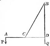
Let ACB be the lever, having AC = a, and CB = 2a. The angle  $ACB = 120^{\circ}$ , and  $BCD = 60^{\circ}$ , and  $CBD = 30^{\circ}$ .
